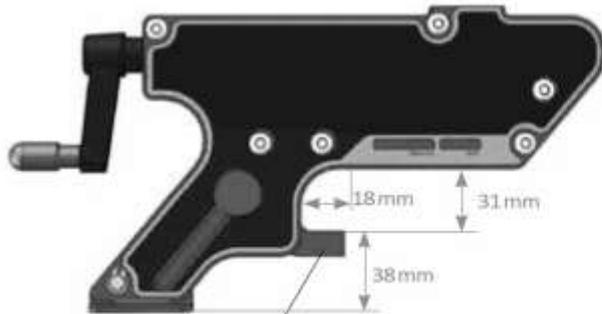
Minimum applicable Bolt Hole Diameter 16mm (0.63")
